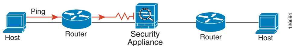
Figure 77-5 Ping Failure Because the Adaptive Security Appliance is Not Translating Addresses
