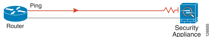
Figure 77-2 Ping Failure at the Adaptive Security Appliance Interface
