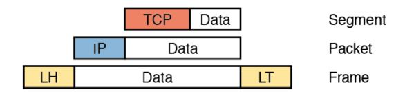
The letters LH and LT stand for link header and link trailer, respectively, and refer to the data link layer header and trailer.
