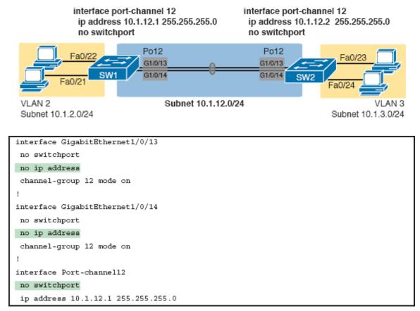
• The figures show an example of the configuration of Layer 3 EtherChannel for SW1.
