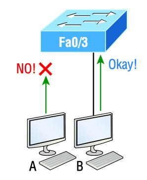
Figure 10.5 shows two hosts connected to the single switch port Fa0/3 via either a hub or access point (AP). Port Fa0/3 is configured to observe and allow only certain MAC addresses to associate with the specific port, so in this example, Host A is denied access, but Host B is allowed to associate with the port.
