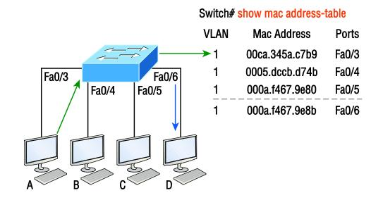
Since Host A's MAC address is not in the forward/filter table, the switch will add the source address and port to the MAC address table, then forward the frame to Host D.
