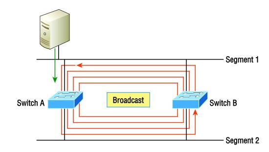
If no loop avoidance schemes are put in place, the switches will flood broadcasts endlessly throughout the internetwork. This is sometimes referred to as a *broadcast storm*.
