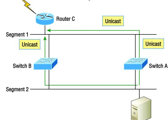
A device can receive multiple copies of the same frame because that frame can arrive from different segments at the same time. Figure 10.8 demonstrates how a whole bunch of frames can arrive from multiple segments simultaneously. The server in the figure sends a unicast frame to Router C.
