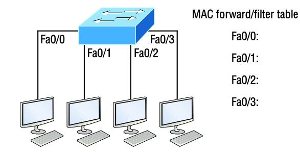
When a switch is first powered on, the MAC forward/filter table (CAM) is empty.
