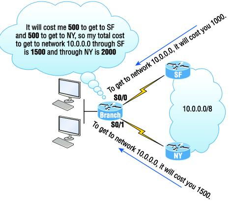
In the figure, the Corp router will have the path through router SF to network 10.0.0.0 in the routing table since it's the lowest feasible distance. It's the lowest true cost from end to end.
