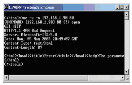
Used to identify a system and services Retrieves information from open ports and services Services respond to banner grabs with application-specific information Can use Telnet of SSH to perform this task
