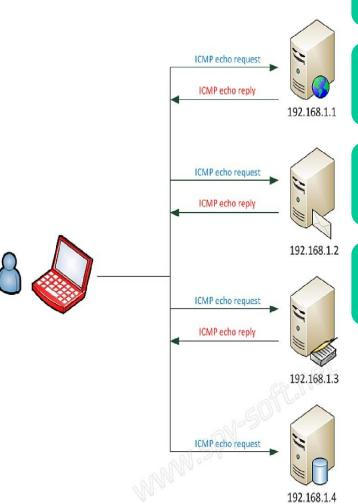
Not every address in a range of IP addresses is "on"
